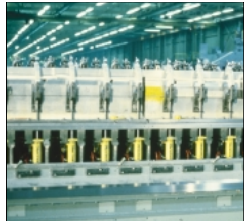
This paper mill uses BRD cylinders for precision when trimming. E
